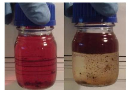
These samples were taken from the same tank before the fuel was cleaned. The left sample was taken from the middle of the tank, the right from the bottom.
