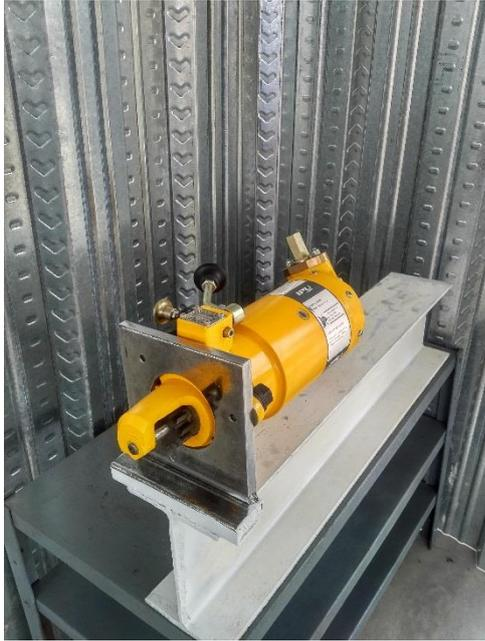
On some applications, the IPU spring starter is being tested while fitted to the storage bracket next to the engine.
